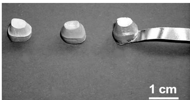
Fig. 1 Plaster stumps for dental crowns. From left to right original stump, stump coated with acrylate dispersion as intermediate layer, and stump prepared as deposition electrode with silver coating and copper ribbon
